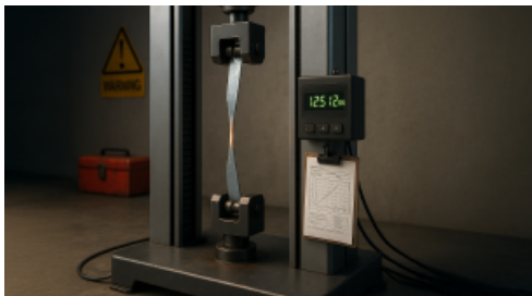
TST (Tensile Strength Test) Determines the maximum load the profile can handle before failure – a critical factor in structural applications.
