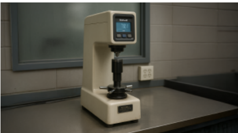
Hardness Test Confirms material hardness to ensure resistance against wear and mechanical damage.
