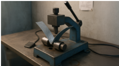
Bend Test Assesses flexibility and the profile's ability to withstand bending without cracking or flaking.
