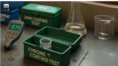
Chrome & Zinc Coating Test Checks the consistency and adhesion of chrome passivation layer applied post galvanization.
